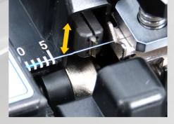
Automatic control of the blade height ensures optimal blade ccondition to and consistent cleave quality.
