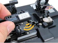
RFID-equipped fibre holder allows the CT110/CT111 to select appropriate cleaving programme.<sup>1</sup>
