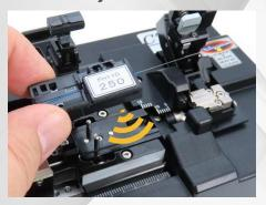
RFID tag equipped to the fiber holder communicate with CT110/CT111 and choose proper cleaving program(\*1)
