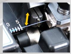
A new blade mechanism controls blade height automatically. It keeps good blade condition to obtain stable cleaving quality.
