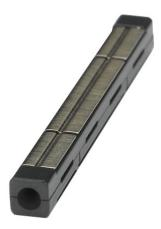
Fujikura's mechanical splice provides an inexpensive, quick alternative to mating fibers. Using V-groove and index matching material technology, this splice maintains both the refractive index and physical contact between the fibers. An assembly tool is used to ensure the fibers are mated correctly. The Fujikura mechanical splice secures both fiber and coating independently with the U-shaped sleeve, enhancing the strength against fiber twist.
